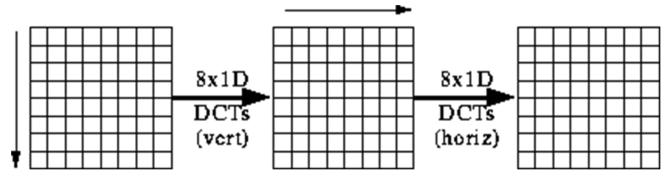
Most software implementations use fixed point arithmetic. Some fast implementations approximate coefficients so all multiplies are shifts and adds.
